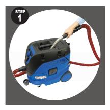
Decontaminate the outside of the extractor by using the extractor.
